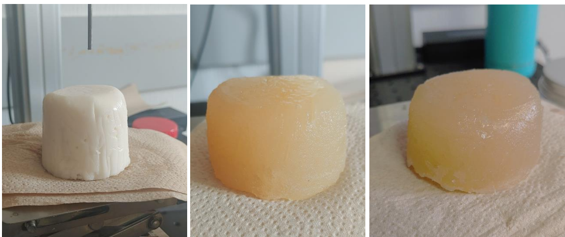
Figure 33. Images of the oil-based phantom (left), Room T PVP phantom (middle) and Fridge PVP phantom (right), after the first measurement.
