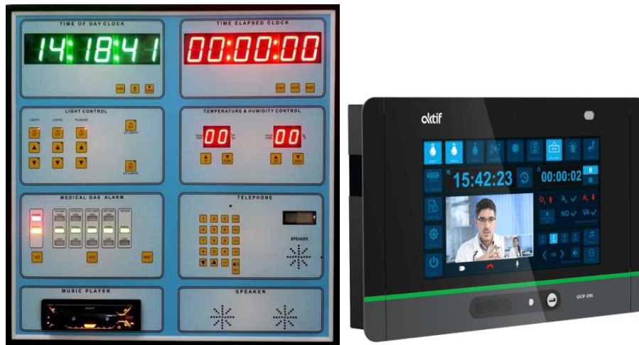
Figure 4. Old generation TCP with modular control systems with buttons (left) and control panel in a touchscreen device, (right). [16, 17].
