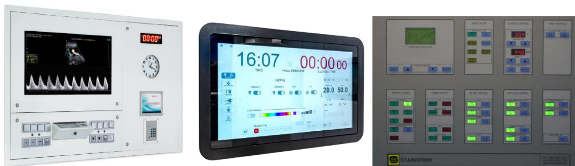
Figure 5. From left to right: Mixed Model (Tedisel), Digital Model (Transforma) and Modular Model (Starckstrom). [27, 28, 26].
