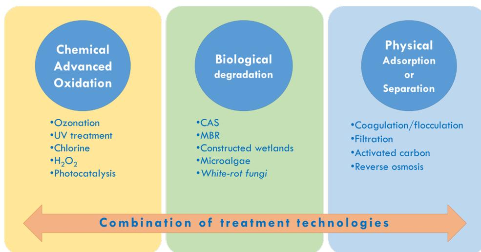
**Figure 1.4.** Scheme of the most typical processes involved in wastewater treatments.
