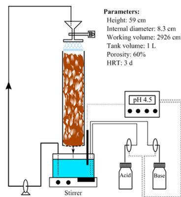
Fig. 1. Schematic representation of the experimental TBR set-up. HRT, hydraulic retention time.
