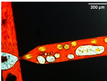
Figure 28. Monodisperse-size formation of unstable 5CB droplets in SSY which finally have the tendency to coagulate.
