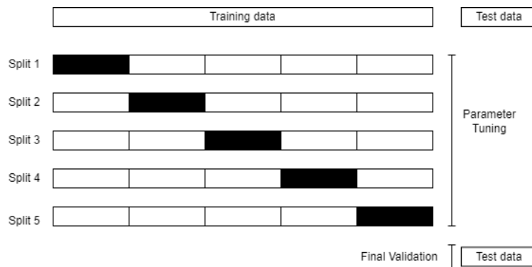
Figure 5.2: 5-fold cross validation schema. Training data is split into 5 folds. In each split black fold represents validation fold and white folds represent training folds.
