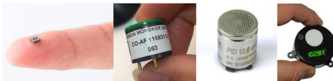
Fig. 3. Examples of low-cost chemical sensors. (From left to right) MOX sensor (Model: Figaro TGS 8100); AGS sensor (Model: Alphasense CO-AF); PID (Model: RAE Systems PID 10.6 eV); (d) NDIR sensor (Model: CozIR by Gas Sensing Solutions).
