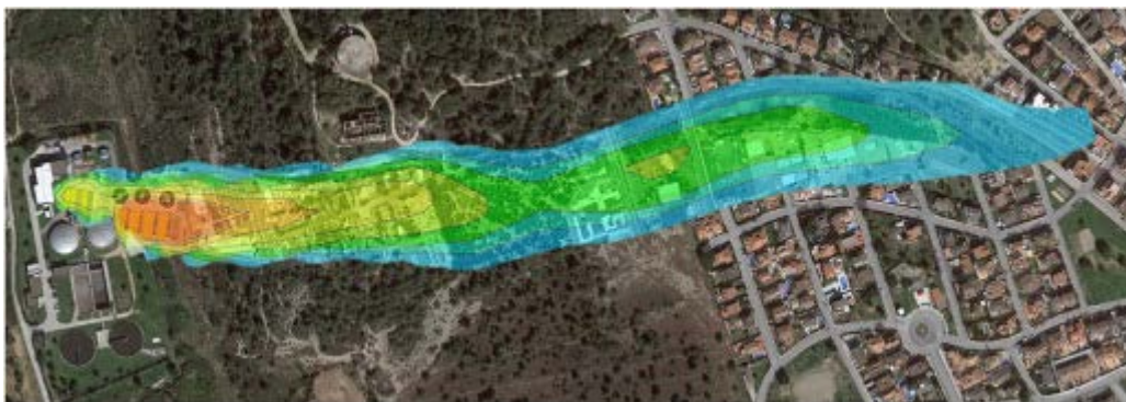
Fig. 11. Time-averaged chemical plume emitted by an industrial site and reaching a nearby population. The plume is simulated using CALPUFF dispersion modelling (Scire et al., 2000). Personal communication from ATTRACT-SNIFFDRONE project.
