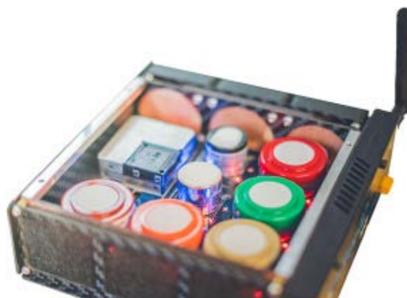
Fig. 4. Commercial multi-sensor unit Sniffer 4D equipped with 5 AGS sensors, 1 PID and 1 NDIR sensor. Copyright Soarability Technologies. Used with permission.
