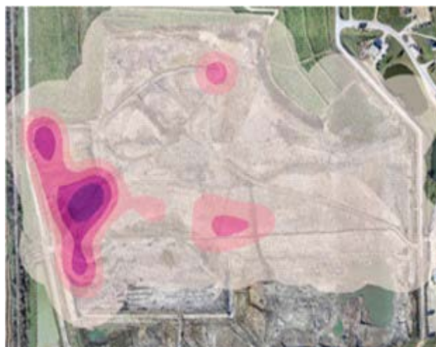
Fig. 17. Surface methane map of a landfill site captured by a RW drone mounting a CP-TDL methane sensor and a 10-m vertical sampling inlet. Permission granted by Sniffer Robotics, LLC.
