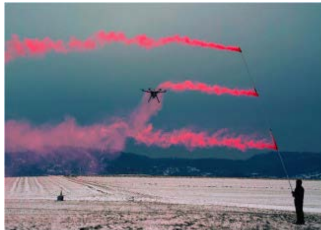
Fig. 2. Downwash of a hovering DJI Matrice 600 drone visualized using colored smoke (Crazzolara et al., 2019).
