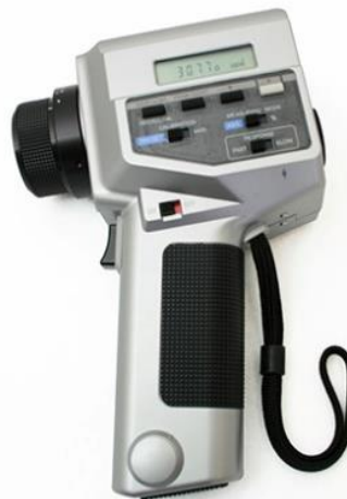
Figure 4 Konica LS-110 for measuring the LEDs.
