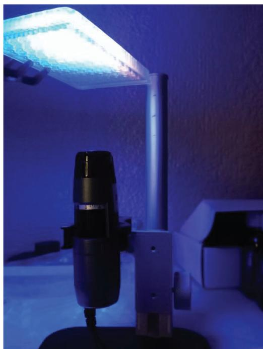
**Figure 14.** A) Rocking shaker. B) Dino-Lite, AM4115TFUW-EDGE digital microscope to inspect microfluidic flow and fluorescence underneath the device.
