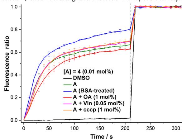
**Figure 4.** Using KCl-KOH assay from POPC vesicles loaded with KCl (100 mM), buffered to pH 7.0 with HEPES (10 mM), different conditions were applied including using BSA-treated lipid, addition of oleic acid at 1.0 mol%, addition of the protonophore CCCP at 1.0 mol%, or addition of valinomycin at 0.05 mol%, on the rate of chloride transport of receptor 4 (0.01 mol%).
