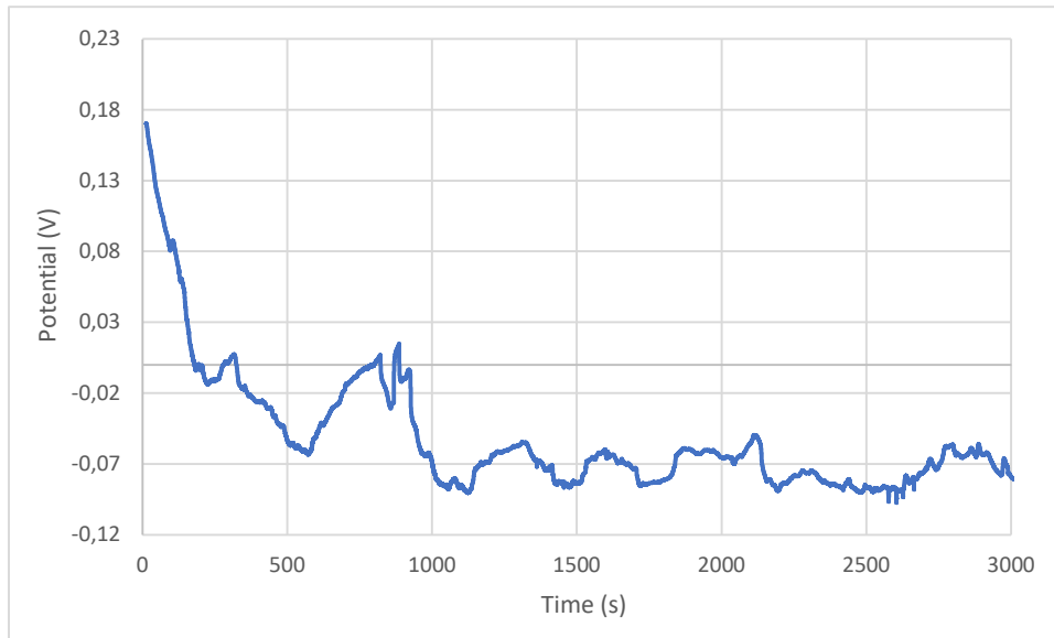
Figure 3.43. Chronopotentiometry of Sensor 10 in 0.1 M KCl.
