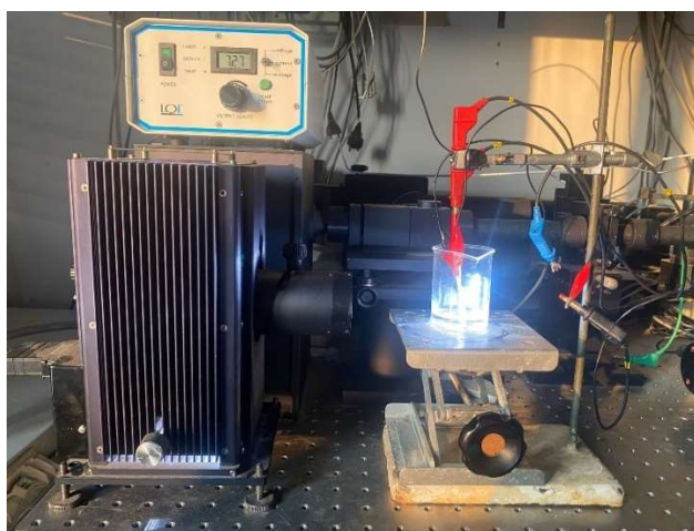
Figure 3.30. Setup employed for light sensing. The sensor is located vertically, with the working area centered in the spotlight.
