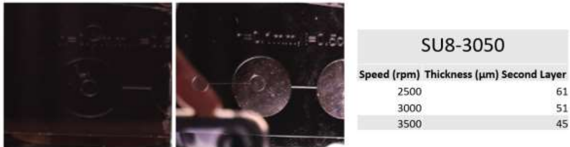
Figure 40. SU-8 3050 optimization of two layers
