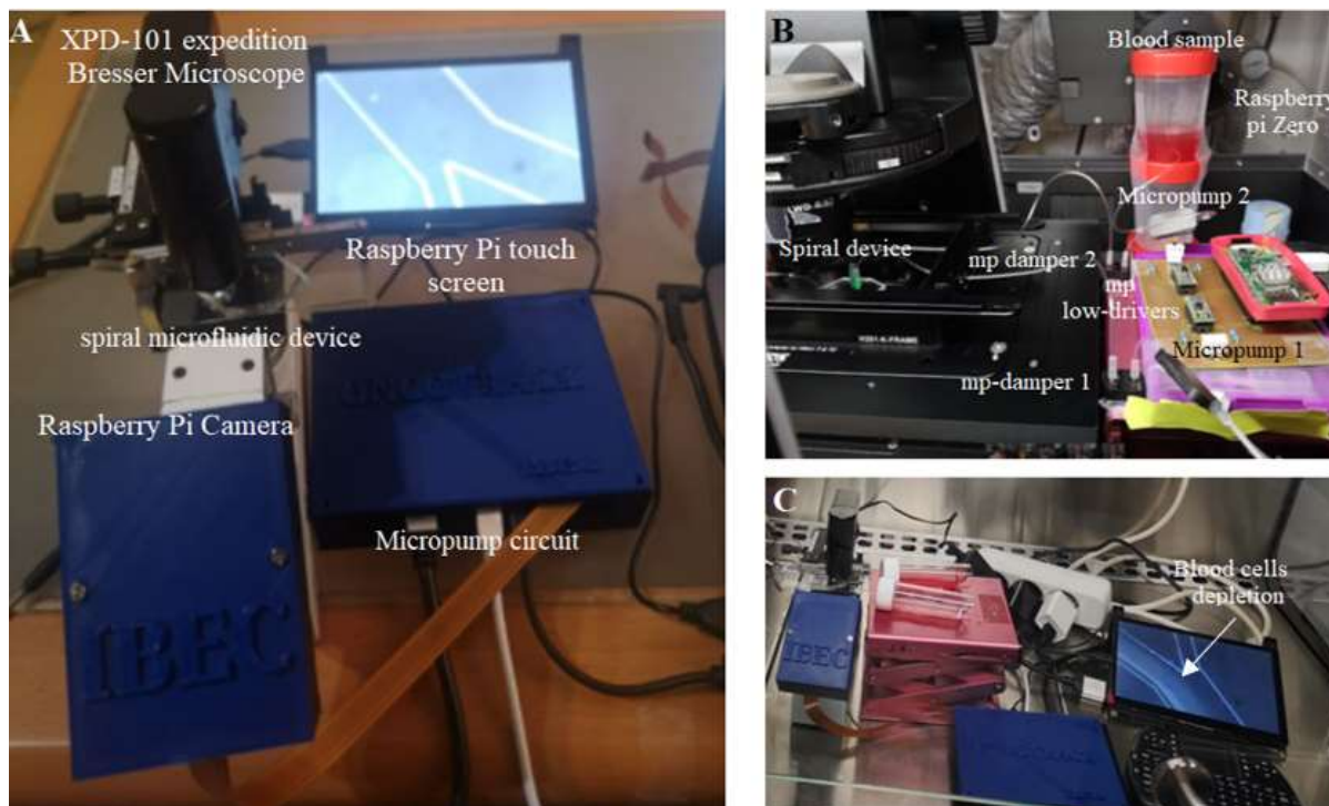
Figure 58. A) Portable biocompatible flow platform composed of Raspberry Pi Camera 12.3MP IMX477 Sensor, micropump circuit, Raspberry Pi touch screen and one small microscope (XPD-101 expedition Bresser). B) Micropump circuit composed of two small micropumps and two mp low-drivers controlled by one Raspberry Pi Zero, two mp dampers and check valves. The system has inlet and outlet reservoirs that can be filled without shutting down the system and allows sample recirculation. C) The depleted blood cells can be recorded and visualized in real time in Bright field.
