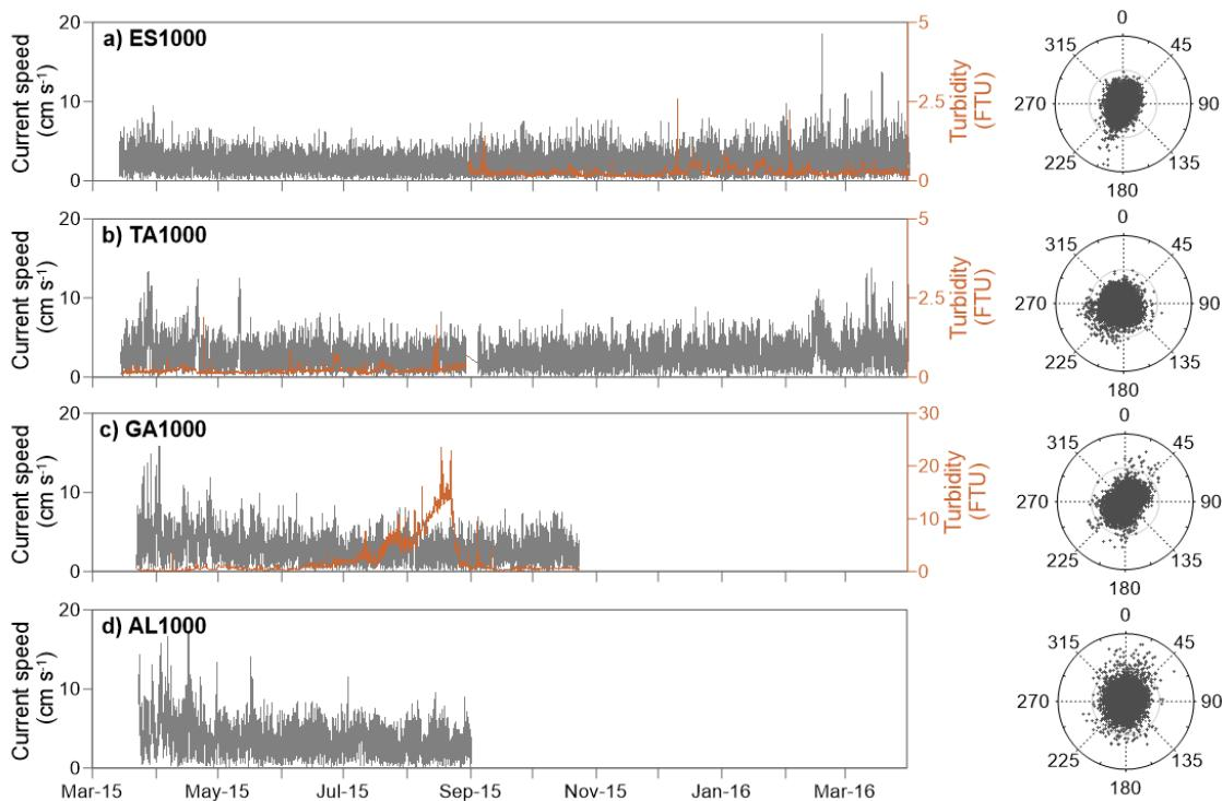
**Figure 3.5.** Current speed (grey line) and turbidity (orange line) recorded at 20 mab in (a) ES1000, (b) TA1000, (c) GA1000 and (d) AL1000 stations. Polar plots show the direction of currents with the X axis ranging from 0 to 20 cm s<sup>-1</sup>. FTU: Formazin Turbidity Units.
