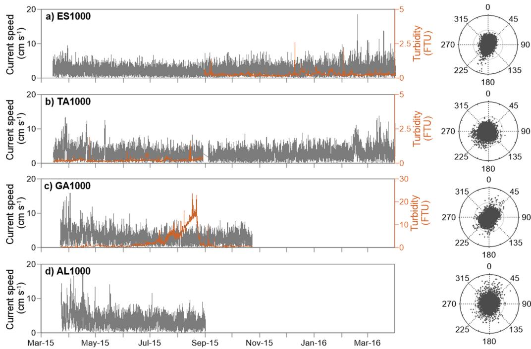
**Fig. 5.** Current speed (grey line) and turbidity (orange line) recorded at 20 mab in (a) ES1000, (b) TA1000, (c) GA1000 and (d) AL1000 stations. Polar plots show the direction of currents with the X axis ranging from 0 to 20 cm s<sup>-1</sup>. FTU: Formazin Turbidity Units.
