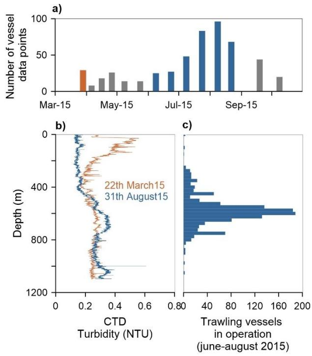
**Figure 3.10.** (a) Number of VSM data points from fishing vessels within a radius of 4 km around GA1000 sailing at less than 5 knots (i.e. while trawling). (b) CTD turbidity profiles performed in March 2015 (orange) and August 2015 (blue). (c) Operating depth of trawling vessels between June and August within a radius of 4 km from the mooring line.
