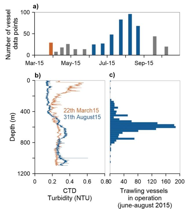
**Fig. 10.** (a) Number of VSM data points from fishing vessels within a radius of 4 km around GA1000 sailing at <5 knots (i.e. while trawling). (b) CTD turbidity profiles performed in March 2015 (orange) and August 2015 (blue). (c) Operating depth of trawling vessels between June and August within a radius of 4 km from the mooring line.
