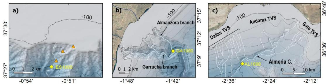
**Figure 3.2.** Bathymetric maps of the heads of (a) Escombreras Canyon, (b) Garrucha-Almanzora Canyon system, and (c) Almeria Canyon and tributary valley systems (TVS). Yellow diamonds show the location of mooring stations and CTD deployments. Orange triangles illustrate a CTD transect across the outer Mazarron shelf and upper Escombreras Canyon. Yellow diamonds indicate the mooring sites.
