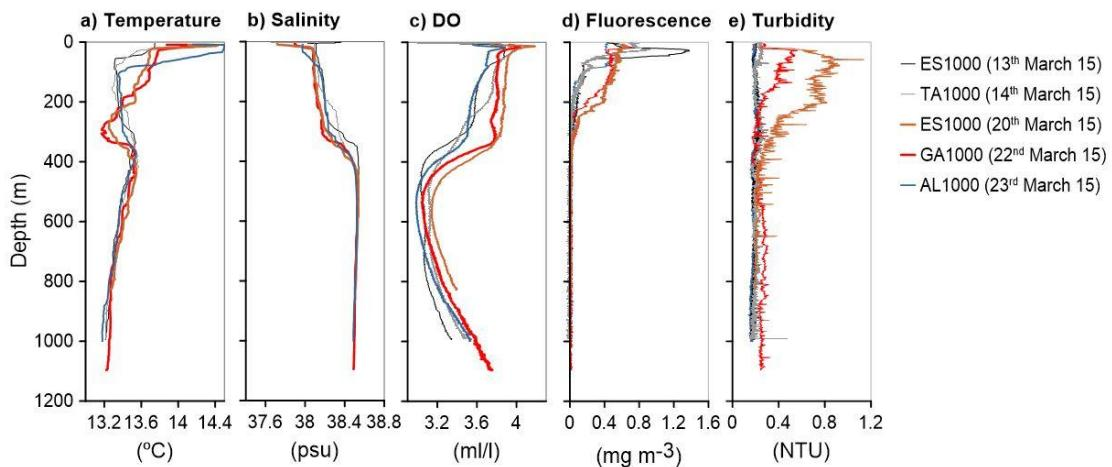
**Figure 3.8.** Hydrological parameters (potential temperature, salinity, dissolved oxygen (DO), fluorescence and turbidity) from CTD transects during mid-March (pre-storm event; grey tones) and late March 2015 (post-storm event; red, purple and blue colours) at ES1000, TA1000, GA1000 and AL1000 stations. Note that AL1000 station is quite far from the rest of stations (Fig. 3.1).
