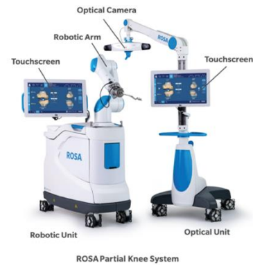
Figure 8. Representation of ROSA Surgical System by Zimmer Biomet.
