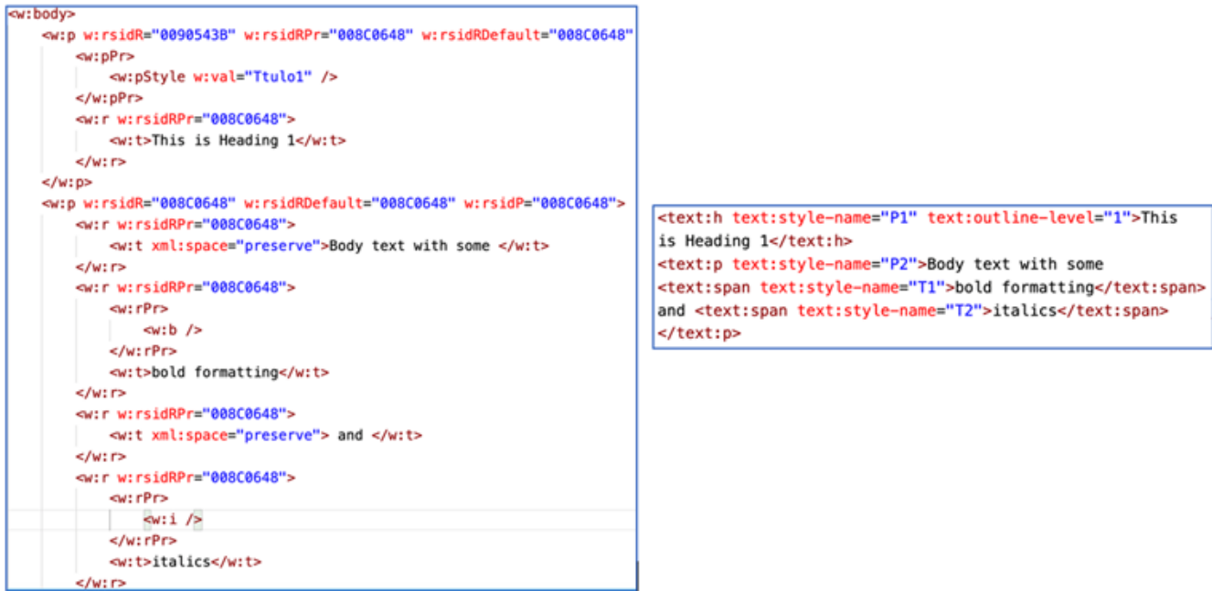
Figure 2: Text and heading in format OOXML (left) and text and heading in format ODF (right).
