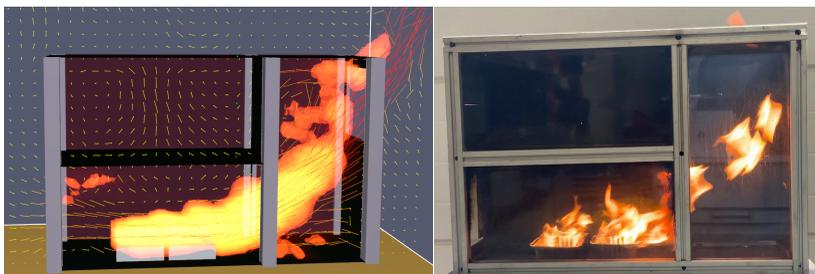
Figure 4.3. Visualization of the unidirectional fire in FDS and real images
