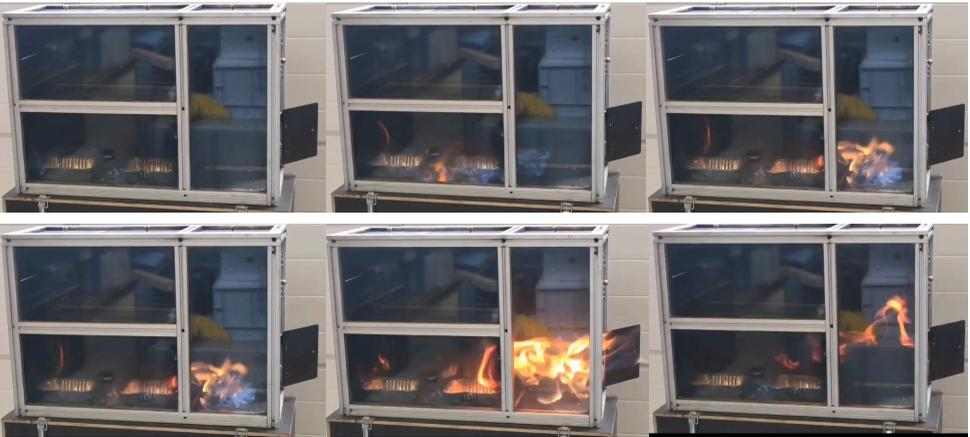
Figure 4.6. Sequence of the backdraft simulated in the scale model
