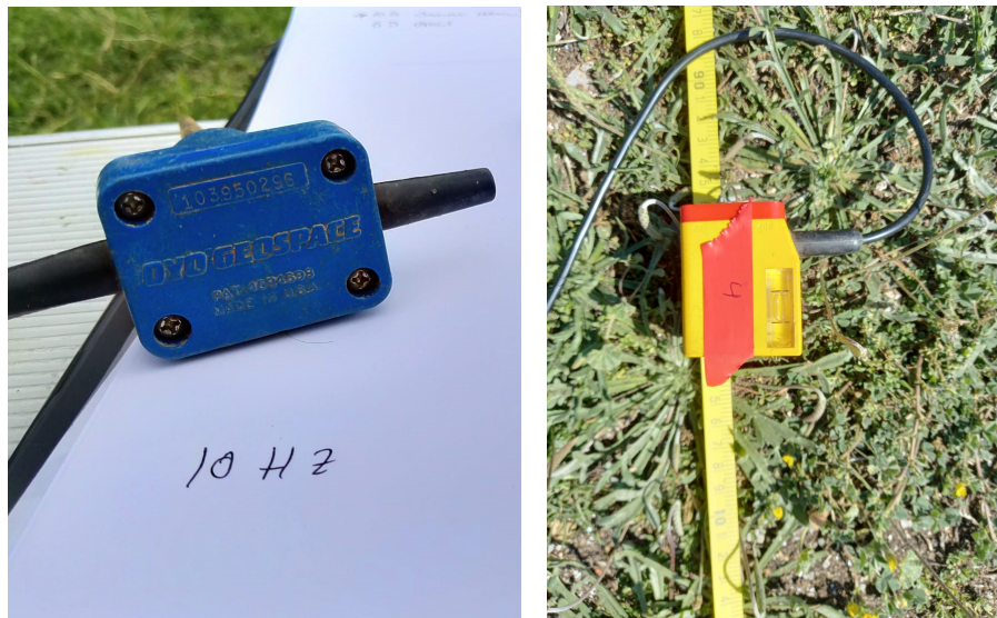
FIG. Appx.1: Image of a P-geophone, of natural frequency 10 Hz, (left); and an S-geophone, of natural frequency 5 Hz, (right) that we used in our survey.
