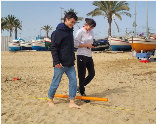
FIG. 2: Photography during the surveying of Platja dels Gossos, with the CMD Mini Explorer device.
