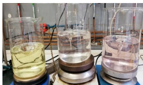
Figure 4. The three pH media after 1 h and 15 min. Left: pH 1.2 medium. Middle: pH 2.2 medium. Right: pH 4.5 medium.
