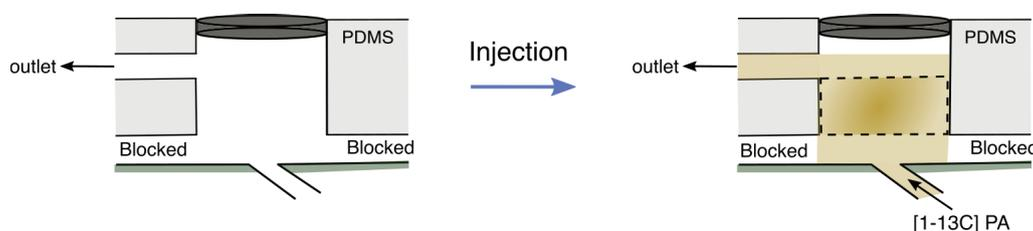
Figure 6.4: Schematic representation of the procedure performed to inject the dissolution inside the microfluidic device through the hyperpolarization channel and filling up the well. In this case I blocked two of the channels to have only one inlet and one outlet. The dashed line in the right figure remarks the physical position of the saddle coil.
