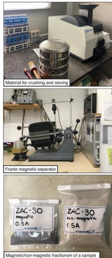
Figure 8. Pictures of the laboratory physical separations.
