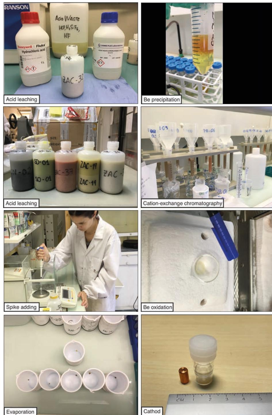
Figure 9. Pictures of the different steps in the chemical separation process. Source: own elaboration.
