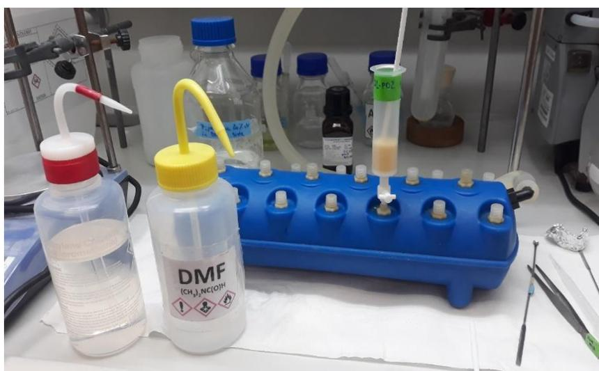
**Figure 4.1** Manifold vacuum ensemble for peptide synthesis in a syringe.
