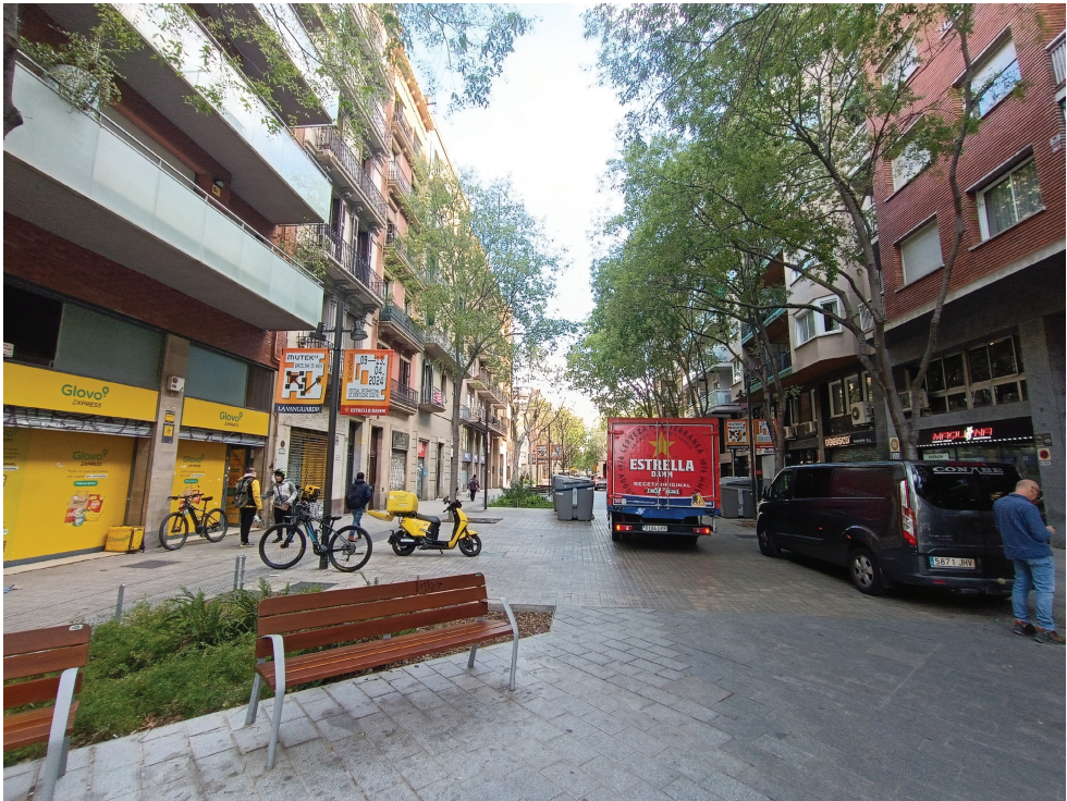
FIGURE 4 The winning project for upgrading the Consell de Cent as part of the Superblock Barcelona project had to be adapted for uses that were not considered in the original design. These modifications included goods loading areas, placement of garbage containers, parking spaces for delivery vehicles, and bar and restaurant terraces. The resulting landscape contrasts with the initial rendering (photo by Lluís Frago, October 2023)
