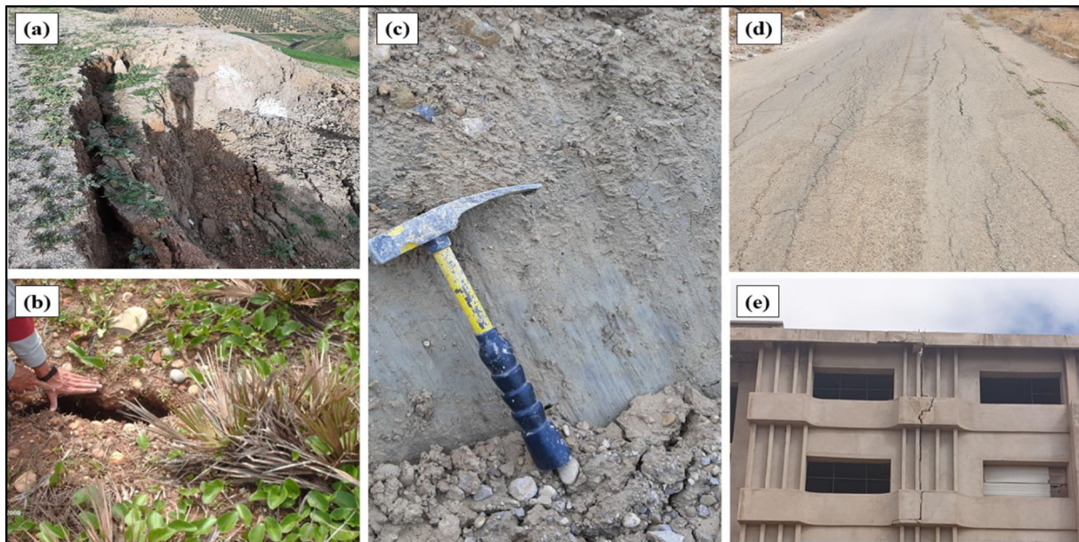
Figure 2. Photographs of different structures exposed in the area. (a) Landslide occurrence, (b) wide (30 cm) and deep cracks in the glacial deposits, (c) fresh sliding surface, (d) severe alligator-shaped cracking, and (e) visible cracks on new constructions.
