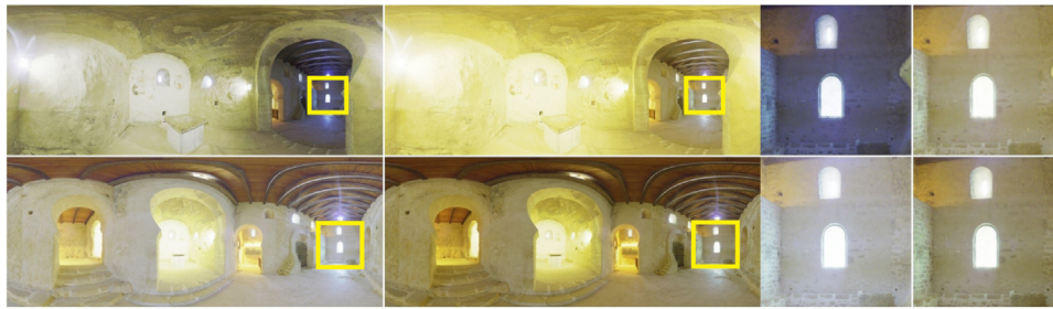
Fig. 4. Gain compensation example. The first column shows a pair of HDR panoramas, which have been uniformized with our approach (second column). Although we removed the effect of color balance (the central apse on the upper row had a strong yellowish illumination), we achieve a much more uniform color across scans. For example, the same wall appears with different brightness levels in the original panoramas (third column), which would lead to visual artifacts if the point clouds are rendered simultaneously. Our approach though achieves more uniform color (fourth column).
