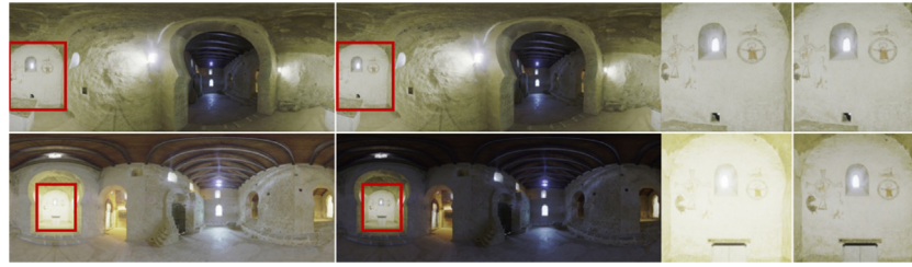
Fig. 16. White balance correction example (original panoramas and compensated ones) focusing on the central apse. Gain factors were optimized taking as reference scan 20 (outside the apse) but here we applied them taking as reference scan 04 (inside the apse), i.e. we applied gain factors \lambda_{q_i}^c / \lambda_{q_{04}}^c instead of \lambda_{q_i}^c . The white balance improvement can be seen by comparing the last column to that in Fig. 13.
