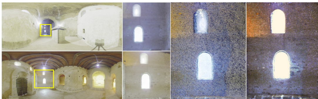
Fig. 3. Laser scanners apply automatic image enhancement techniques to individual panoramas (left). In challenging scenes with varied illumination profiles, the same surface (e.g. the highlighted wall) may appear with very different colors/brightness depending on the scan (middle left). Since these images are used to color the point samples, rendering simultaneously multiple registered scans (middle right) produces severe visual artifacts, with pseudorandom patterns according to the visibility of the points from the different scans. Using HDR images and advanced tone mapping techniques (rightmost image) does not solve the problem.
