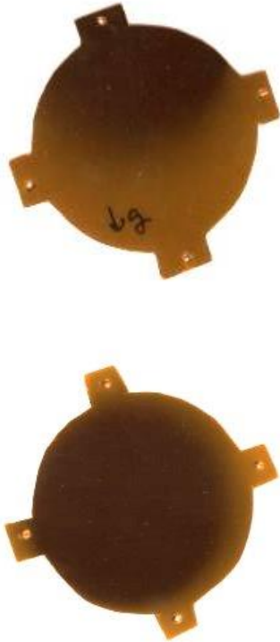
Fig.3 Misalignment analysis procedure. 1: Film is scanned 2: Two circles of the size of the collimator and disc are superimposed to the image. 3: distance between the circles is determined. In the cases where gravity direction is registered, the parallel and perpendicular components are also registered. 4: From the two circumferences radius and the distance between the centers, the superposing area can be derived.
