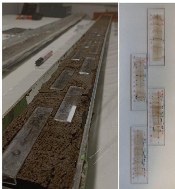
Fig. 3.3: Thin sections: a) Sampling sediments for thin sections. b) Laminated pattern and marker layers identified in the thin sections.
