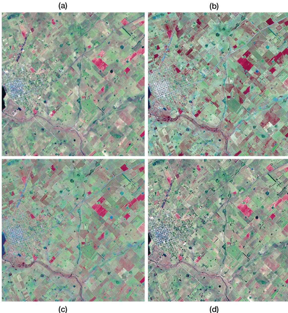
Fig. 2. (a) Detail of the Landsat (TM) image, (b) Result of fusion by the standard IHS method, (c) Result of fusion by the standard LHS method, (d) Result of fusion by the AWL method.
