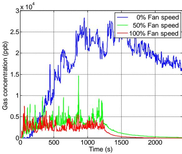
Fig. 10. Gas evolution at spatial point 1 obtained for different fan speed levels.
