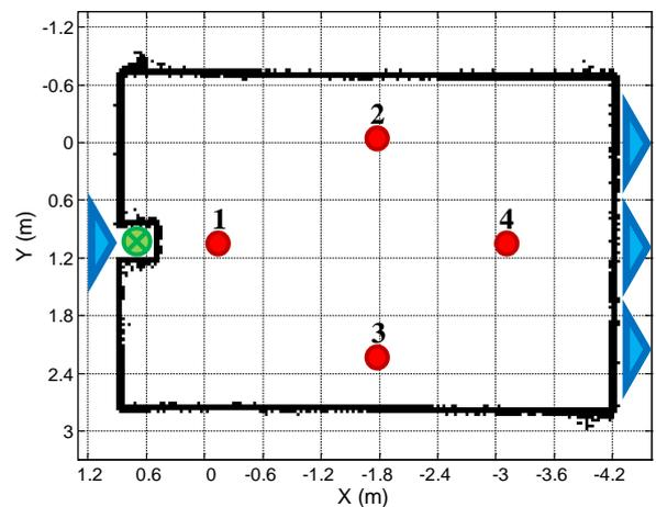
Fig. 3. Wind tunnel map with fans (blue triangles), gas source (green circle) and static measurement points (red circles).
