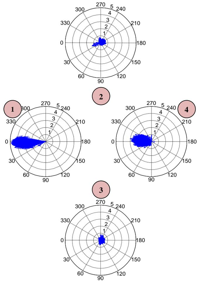
Fig. 8. Wind intensity and direction (m/s) at the four static measurement points defined in the case of fans at full speed. The direction depicts the precedence of the wind.
