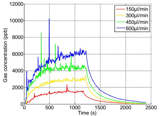
Fig. 6. Static measurement: gas evolution measured at point 3.
