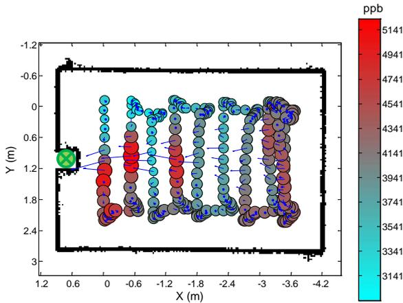
Fig. 11. Final sampling with a semi-random robot exploration.
