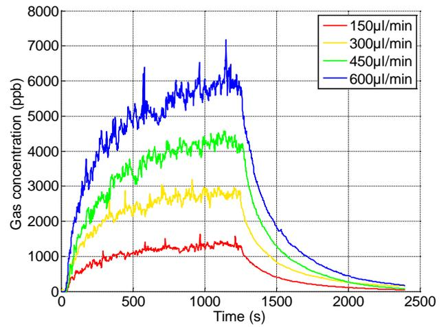
Fig. 5. Static measurement: gas evolution measured at point 2.
