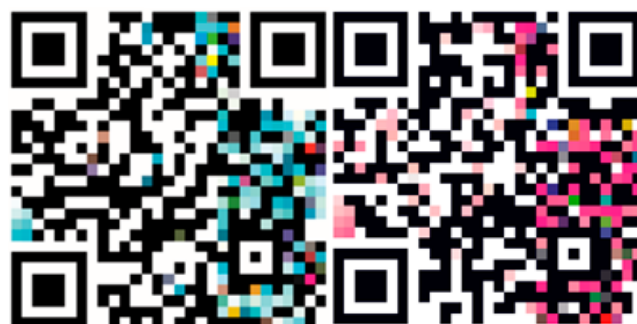
Figure 2. (a) QR codes designed for use with Sensafe® chlorine test strips and (b) the DPD method (right). The QR codes encode a URL to the Diesmar website and contain a color palette for color correction. The specific URLs encoded are: (a) http://diesmar.com/#AdDk (accessed on 18 May 2025) and (b) http://diesmar.com/#n87RXv6i3 (accessed on 18 May 2025).
