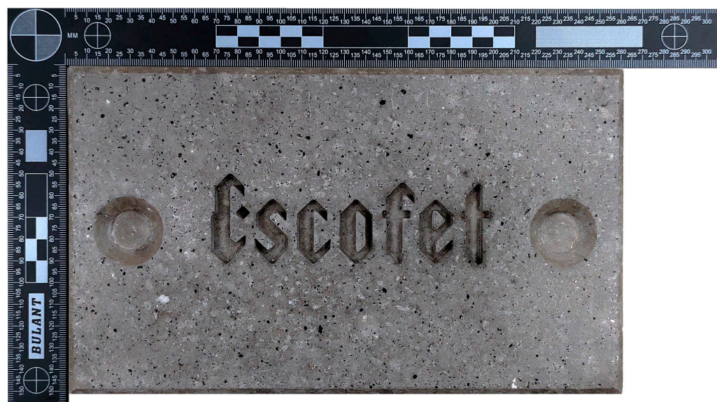
Figure 6. Cast concrete paver formulated from an alkali-activated binder using incineration bottom ash (IBA) as the sole precursor, and granitic aggregates.
