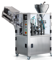
Figure 15. Automatic filling and sealing machine (PK-01).
