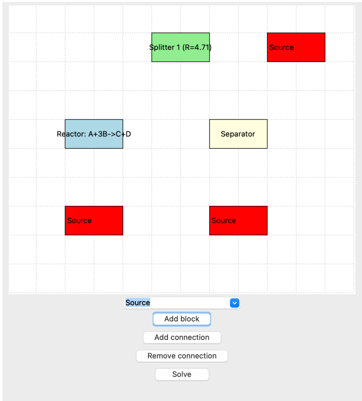
Figure 8. Insertion of process blocks into the flow diagram using the graphical interface.
