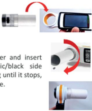
Remove the wrapper and insert the turbine (plastic/black side first) into its housing until it stops, then rotate clockwise.
