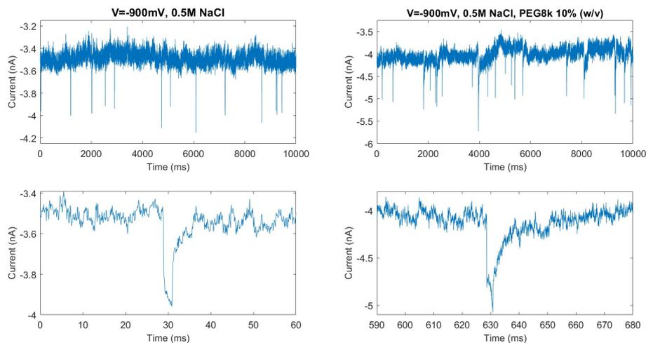
FIG. 5: Ionic current measured in 0.5 M NaCl solution with and without PEG 8k 10% (w/v) in the central chamber. A single translocation event sample for each case is shown below.
