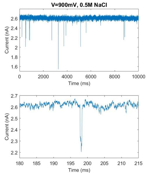
FIG. 4: Ionic current measured in 0.5 M NaCl in the central and lateral chambers, for 900 mV applied to the nanopipette. A translocation event is shown below.
