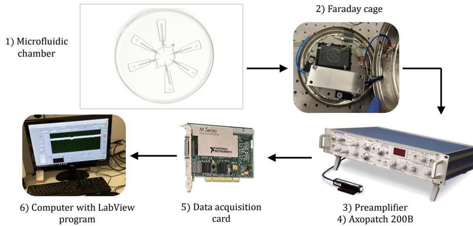
FIG. 1: Schematic representation of the microfluidic chamber and the electrical setup used for the translocation experiments.
