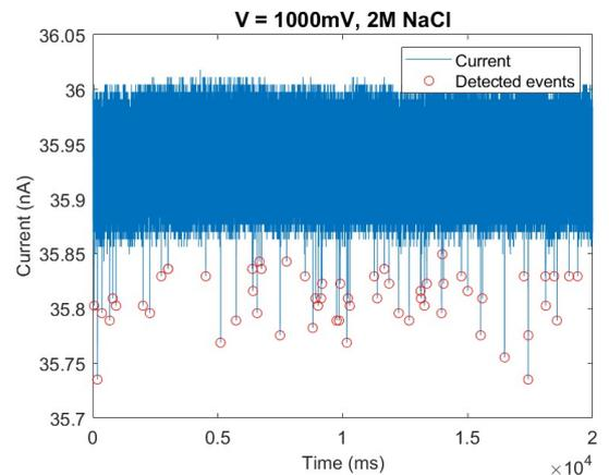
FIG. 3: Ionic current measured in 2 M NaCl solution for 1000 mV applied to the nanopipette. The downward peaks circled in red represent the dsDNA translocation events found with the Matlab algorithm.
