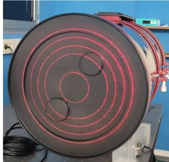
Figure 6: Projection from the emitter telescope onto the covered receiver telescope, showing concentric ring formation with the guiding laser (2" collimator, Howie Glatter).
