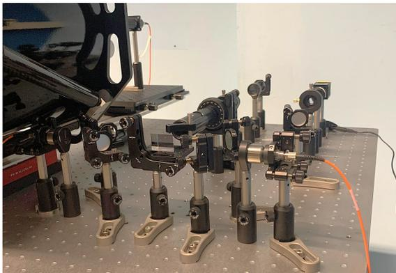
Figure 7: Experimental set-up of the entangled-photon collection.
