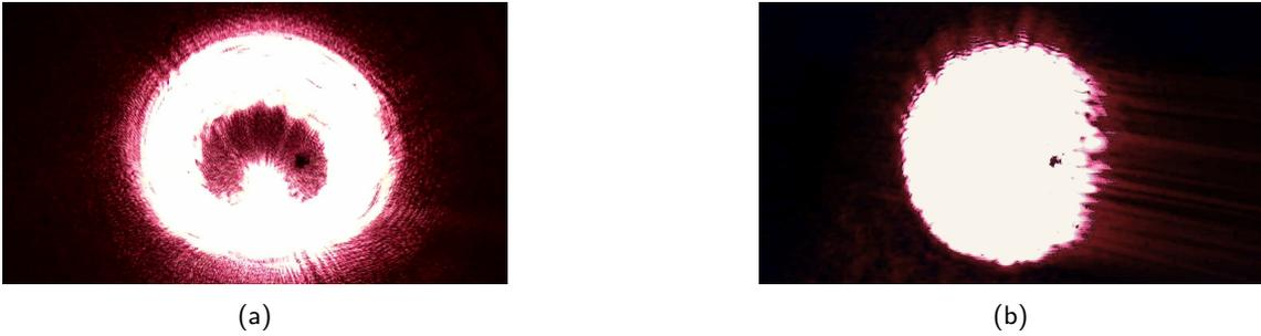
Figure 14: Beam images captured at the receiver using a CMOS sensor. (a) Beam at the telescope focal plane using the axicon configuration. (b) Beam profile using the displaced beam configuration.
