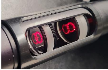
Figure 5: Ring profile observed at the second axicon output and at the achromatic lens using a fiber-coupled alignment lamp (VLP50, NetPeppers).
