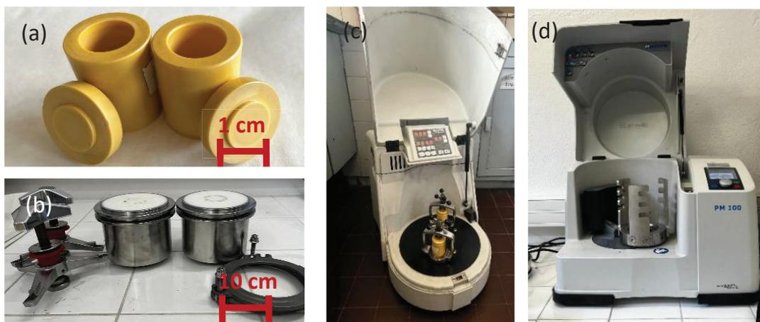
Figure 4.1. Jar pots of (a) sBM and (b) bBM and (c) ball milling sBM and (d) ball milling of bBM equipment.
