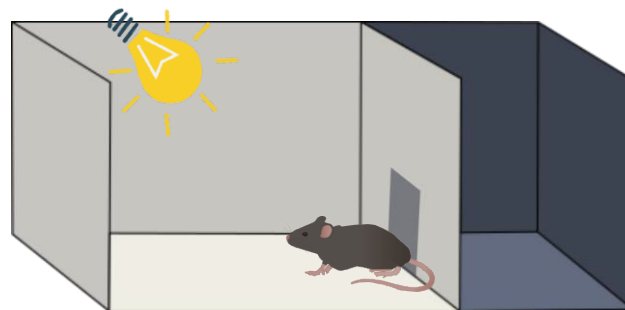
Figure 22. Schematic illustration of the dark-light apparatus. The latency to cross from the dark compartment (right) to the light compartment (left) was measured.
