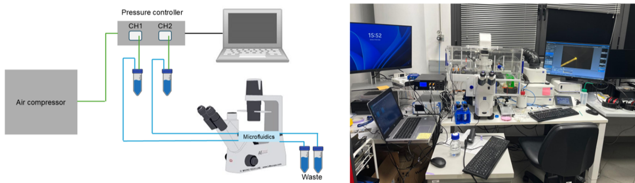
FIG. 6: Supplementary 1. (a) Schematics of the experimental setup. Green lines represent air connections, blue lines represent liquid connections, and black lines represent electrical connections. (b) Photograph of the experimental setup.
