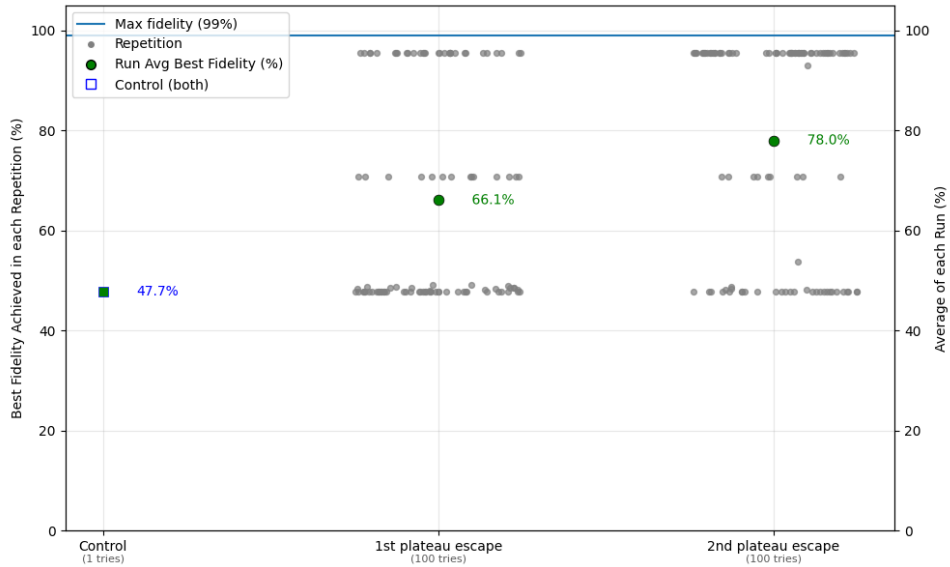
Figure 5.5: Two trapped plateaus at 47.7% fidelity escape when adding a randomly initialized ancilla qubit in “bridge” topology, showing in gray the best fidelity F_{best} in each repetition (100 each), and in green the average F_{avg,best} .
