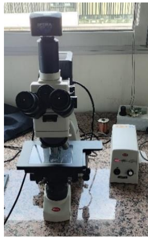
FIG. 7: An image of the optical microscope (left) as well as the source of light used to illuminate the samples from above (right).
