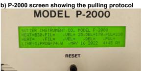
Figure A.2: **P-2000 pipette puller.**a) Image of the P-2000 pipette puller from Sutter Instruments. b) Screen display showing the parameters of the protocol used to pull nanopipettes with a tip diameter of 10-50 nm.
