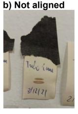
Figure A.3: a) The pattern on the laser paper when the pipette puller laser is properly aligned and centered on the glass capillary. b) Pattern when the laser is misaligned.
