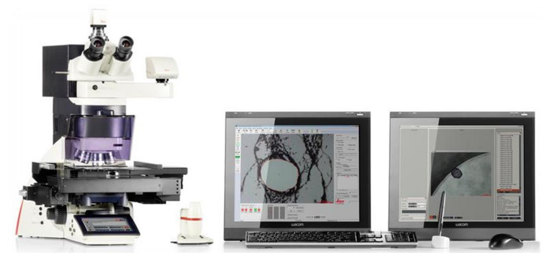
Figure 37. Image showing the Leica Laser Micro-dissection system.
