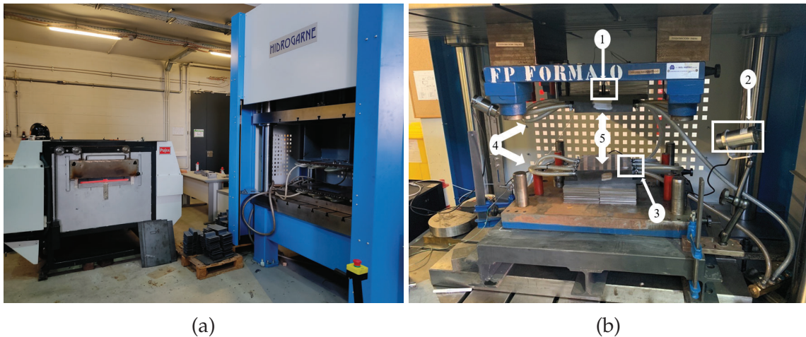
Figure 7.2: (a) The pilot plant at Eurecat Manresa where the tests have been performed. The furnace is located on the left-hand side of the image and the hydraulic press that contains the die is on the right-hand side. (b) Cooling die with cooling channels inside the hydraulic press. Localization of the three temperature sensors in the setup. 1) S1. 2) S2. 3) S3. 4) Cooling channels. 5) Cooling die.
