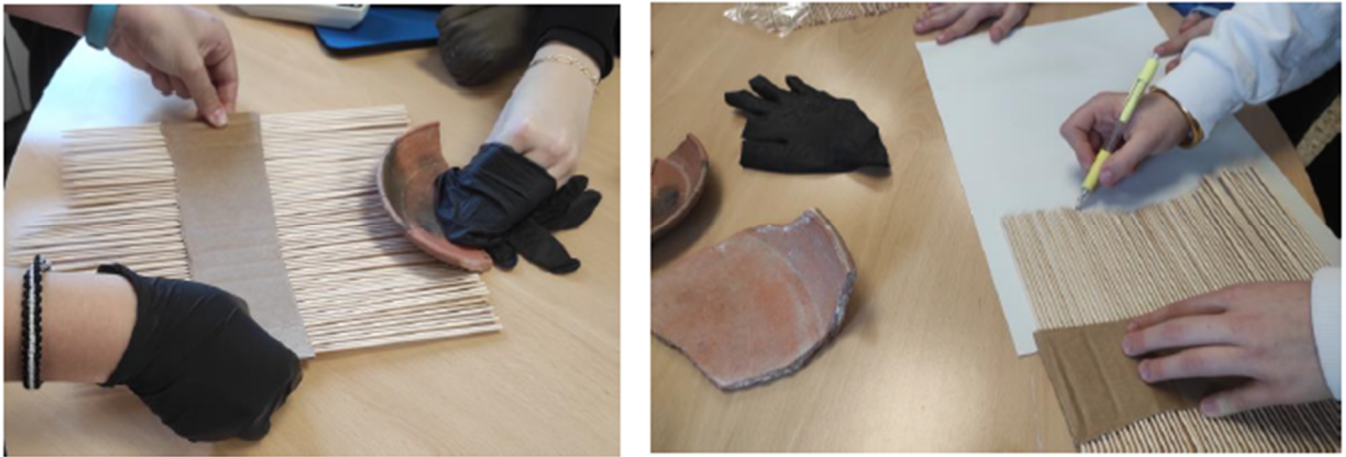
Figure 3. Teacher's observation of the students using the profile gauge to obtain the contour of a section of one of the ceramic pieces. Authors' archive.
