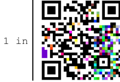
Fig. 1: A back-compatible Color QR Code for the evaluation of colorimetric indicators. This QR Code is read by commercial scanners and should display the URL: c-s.is/#38RmtGVV6RQSf , includes up to 125 reference colors and the colorimetric dye is printed above the lower finder pattern, represented here as seven purple modules.
