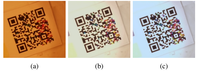
Fig. 4: A printed machine-readable pattern featuring a Color QR Code and a colorimetric indicator inside the sensor chamber. The image shows the Color QR Code before exposure to the target gas under three different light conditions: 2500 K (a), 4500 K (b), and 6500 K (c).
