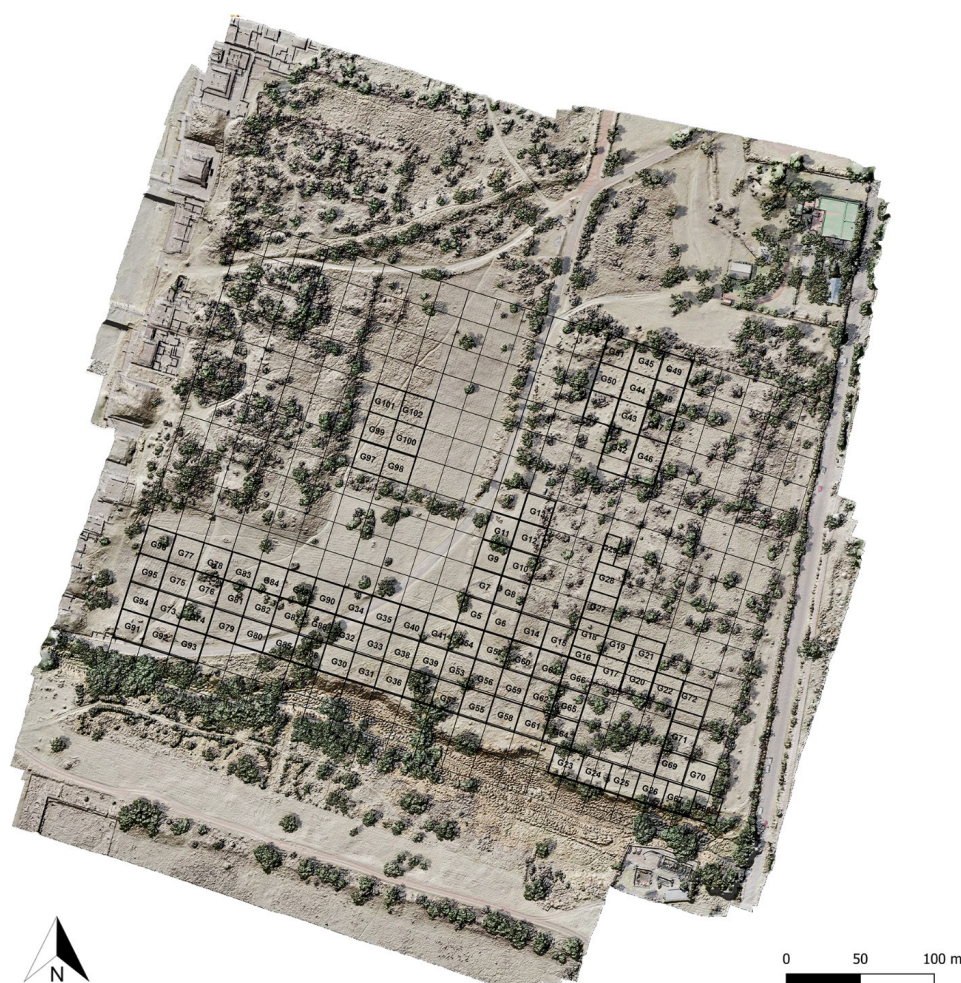
Figure 2: 20x20 grid units used for magnetic gradient survey in N2E1 quadrant. The recording of surface materials was carried out following the same grid, although not all the squares of the grid west the Street of the Dead, to the south the San Juan river.
