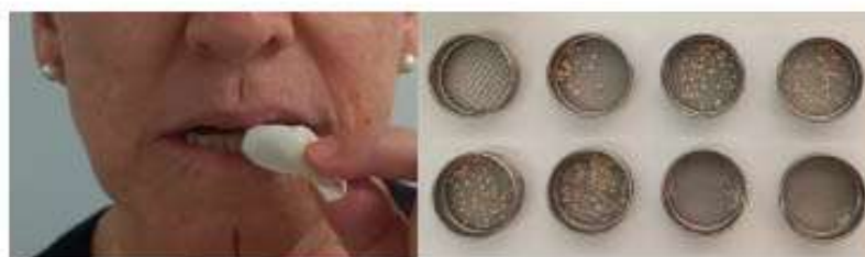
Figure 1. Participant initiating the masticatory assay and particles obtained on each sieve.
