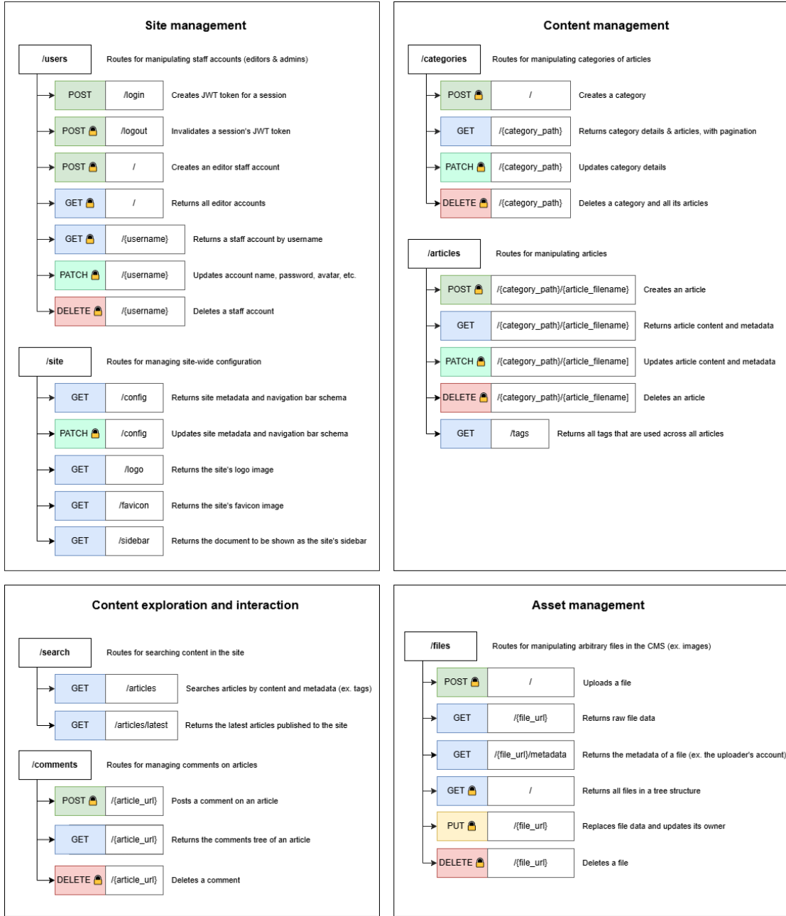
Figure 6: Diagram of the backend's API routes, indicating the endpoints and methods they accept. A lock icon indicates endpoints that require authentication.
