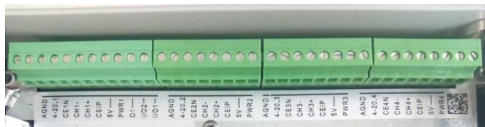
Image 1: Channels and connectors from the analog logger.
