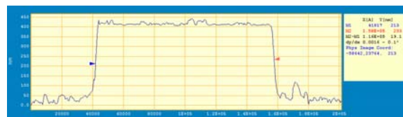
Fig.4. SEM and AFM profile of a rib-loaded waveguide
